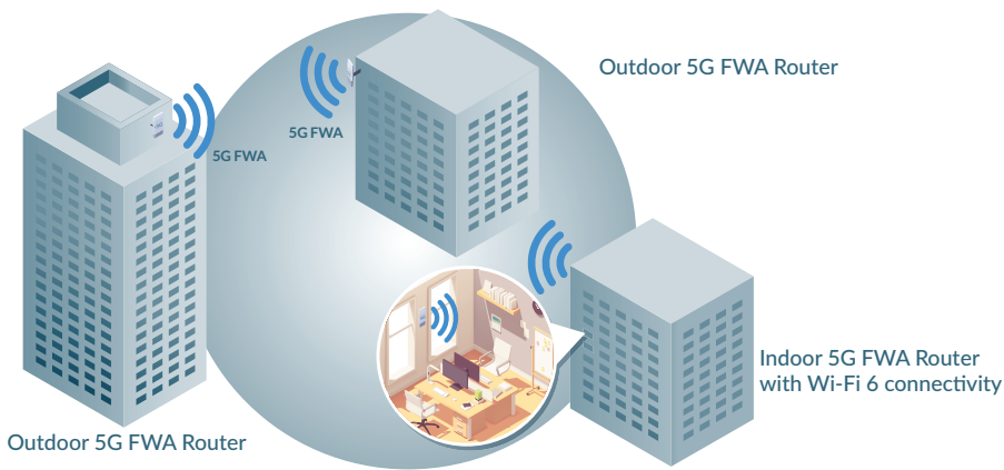
Figure 9: 5G FWA connectivity for a campus private network
